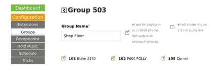
Grandstream, Most Cisco's, HTEK, Atcom... all listen for a multicast RTP audio broadcast on a port, per group.
