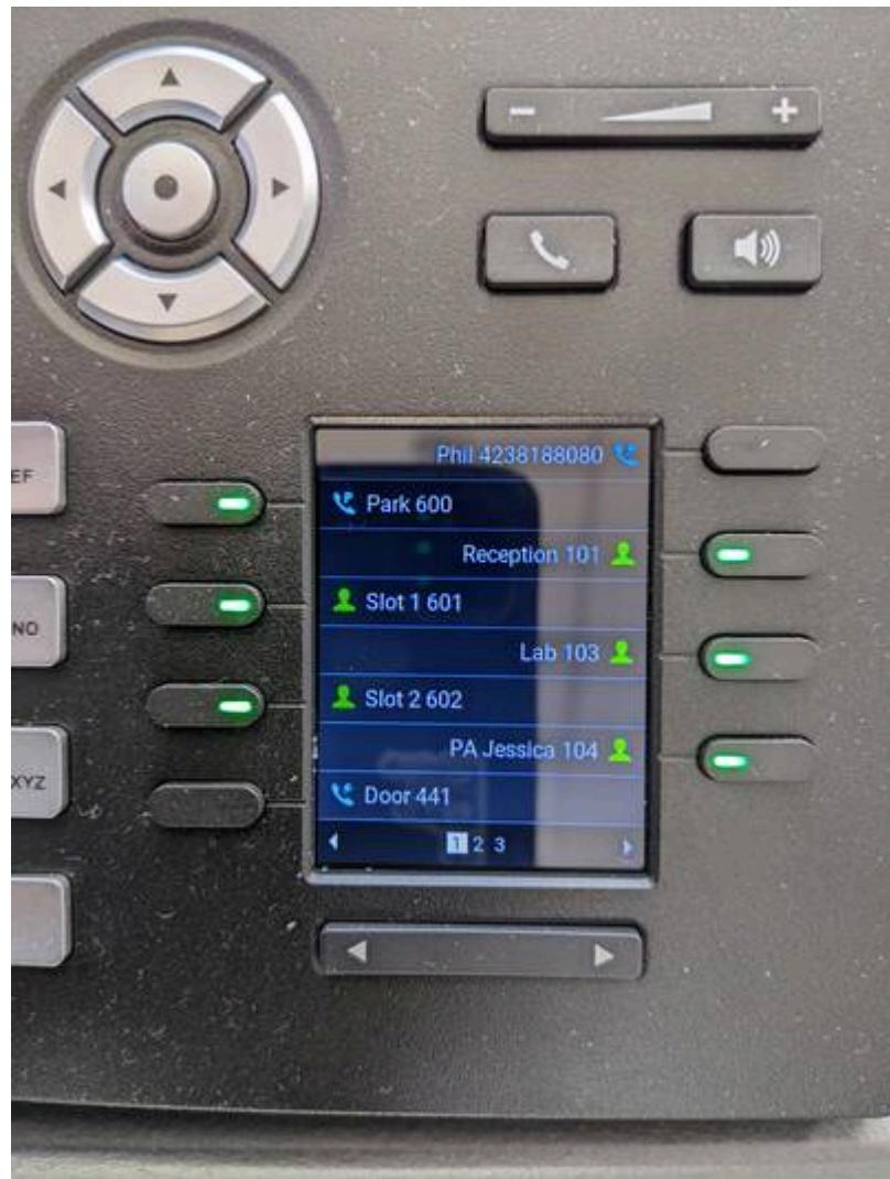
Arguably, this is the feature that makes a business phone system powerful. Ring-U automatically configures “soft” and physical key functionality on all Grandstream phones that support it (GRP2135, GRP2170, GXP2614, GXP2616) with a layout similar to the one in the picture
