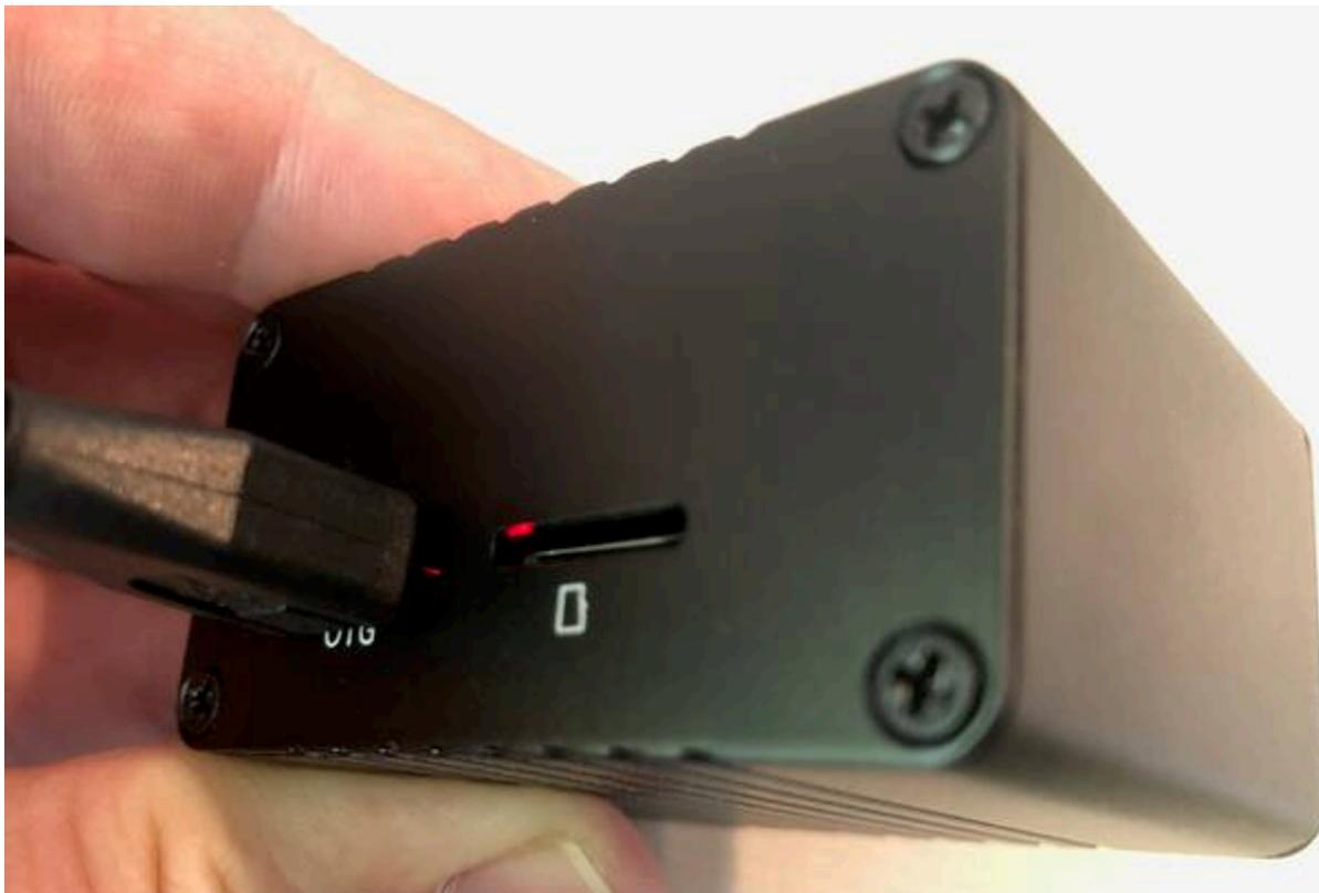
Power light is a pinhole red light next to power supply in. Also visible from SD card slot.
