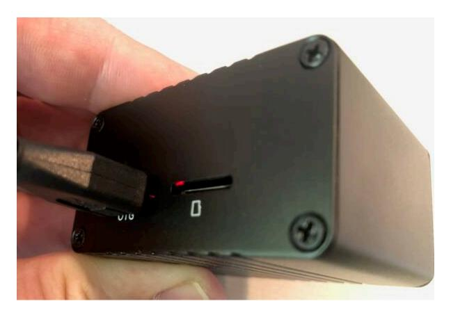
Power light is a pinhole red light next to power supply in. Also visible from SD card slot.
